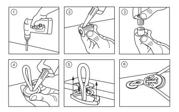
Drill a hole for the double TDP. Clean the installation area with acetone to remove dust and grease. Apply Sikaflex 291i or other adhesive to make the installation watertight. Tighten the double TDP. Attach the SLR to the loop. Wait 24 hours before putting any load on the product.
