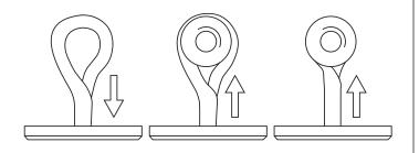
Stretch the loop open and slide in the SLR. Close the loop to lock the SLR in place.
